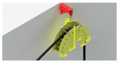
Working position A Hanging block. By means of shackle can be connected to the interference structure or crane.
